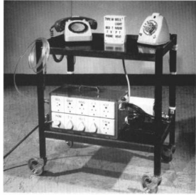
FIG. 3 First general-purpose control console with indicator and load-opening telephone.
